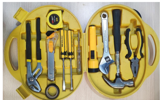
Toolkit for minor repairs and maintenance of sanitation facilities
